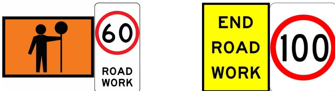
Figure 6-6. Side-by-side dual sign arrangements
